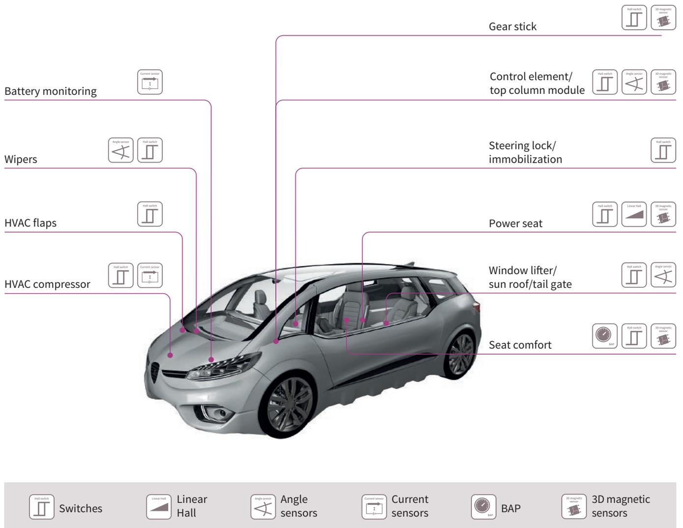
The body segment presents the most diverse target market for sensors. Hall switches, for example, are deployed in classic applications such as window lift modules, whereas
