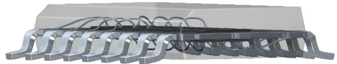
Thanks to the use of innovative stack-mounting technology, the devices of the angle sensor family combine two independent sensors within standard and space-saving TDSO packages which are only about 1 mm thick. It has the same width and length as a conventional single-sensor package. Compared to the common approach of side-by-side sensor placement, the advantages of the top-bottom placement
