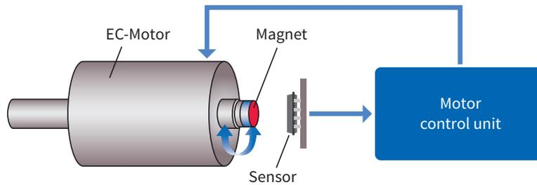
A correct commutation of the EPS motor has to be ensured, in order to avoid a blocked steering or the erratic steering support. This application is also classified in the category of ASIL-D. To achieve this high level of functional safety, Infineon offers angle sensors in the dual-sensor package that allow the integration of two redundant sensors in the place of one.
