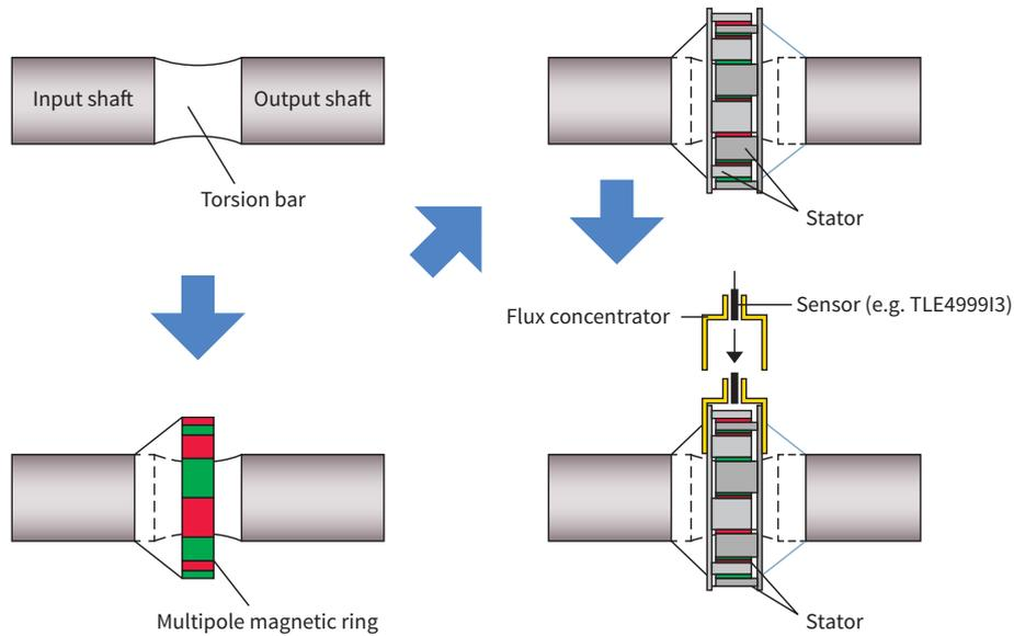
Conventional EPS systems use two linear Hall sensors for ASIL-D compliance have to shut-down in the event of a loss of one sensor signal. Therefore, the trend in EPS systems is to increase availability by implementing additional sensor signals or plausibility mechanisms. To support this trend towards high-availability EPS functionality, Infineon recommends the usage of two TLE4998 dual-sensors or
