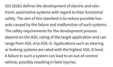
All newly developed parts, which are addressing a certain safety goal will be based on an ISO 26262-compliant development flow, thereby allowing direct use in all safety-relevant applications.
