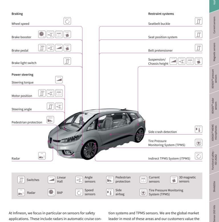
At Infineon, we focus in particular on sensors for safety applications. These include radars in automatic cruise control systems, wheel speed sensors in ABS and ESP features, pressure sensors in side airbags and pedestrian protection systems and TPMS sensors. We are the global market leader in most of these areas and our customers value the outstanding levels of quality and reliability that we deliver.
