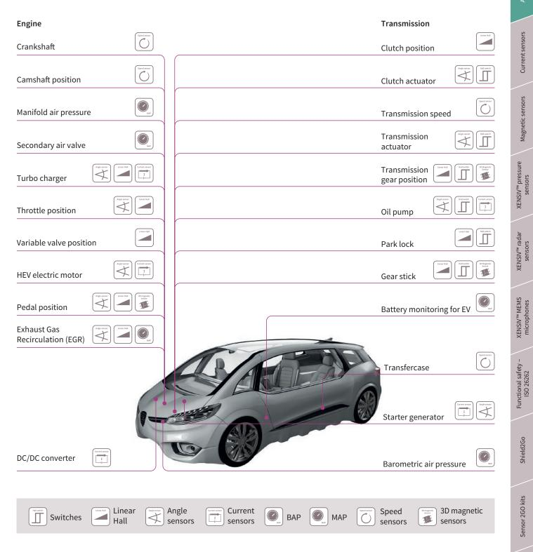
Crankshaft, camshaft and transmission speed sensors as well as MAP and BAP pressure sensors are only some of the key elements of multiple modern powertrain applications, such as engine and transmission, which significantly boost drivetrain efficiency. Our broad portfolio of products fits every customer requirement.
